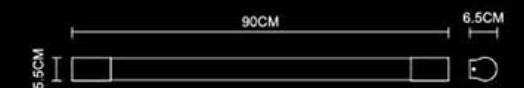
Innervation 900 Wall Lamp 1442 T5 1x21W T5 HO 1x39W Stainless Steel Polished IP44
