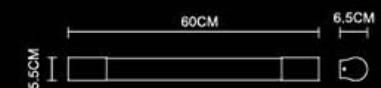
Innervation 600 Wall Lamp 1441 T5 1x14W T5 HO 1x24W Stainless Steel Polished IP44
