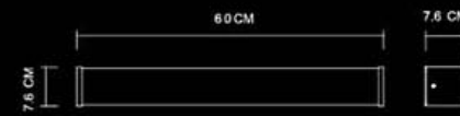
Meteor 600 Wall Lamp 1523 T5 1x14W T5 HO 1x24W Stainless Steel Polished ⊕ IP44
