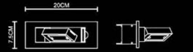
Tank Tank Recessed Wall Lamp-MDC Switch 1670 LED 1x3W Stainless Steel Polished 16CMx5.7CM Hole On The Wall
