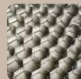
Sandwich Top with Honey comb and Laminate
